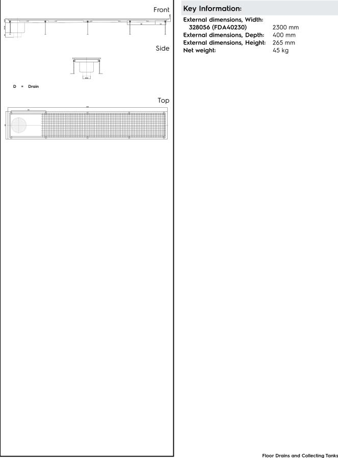
Floor Drains and Collecting Tanks Floor Drain with Stainless Steel Grate and Side Drain - Vertical outlet 400x2300 mm The company reserves the right to make modifications to the products without prior notice. All information correct at time of printing.
